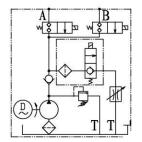
This power unit use no-leak dual way check valve to realize the complete isolation of two lines. It makes this two lines totally independent in the action of lift and fall. It is the ideal hydraulic power for multiple cylinder single lift system. This power unit widely used in primary and big scissors lift.
